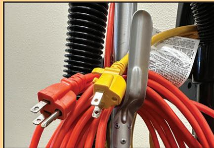
**Can you spot the safety hazard here? The ground prong is missing on this vacuum plug. Replace the plug so it has the third prong.**
