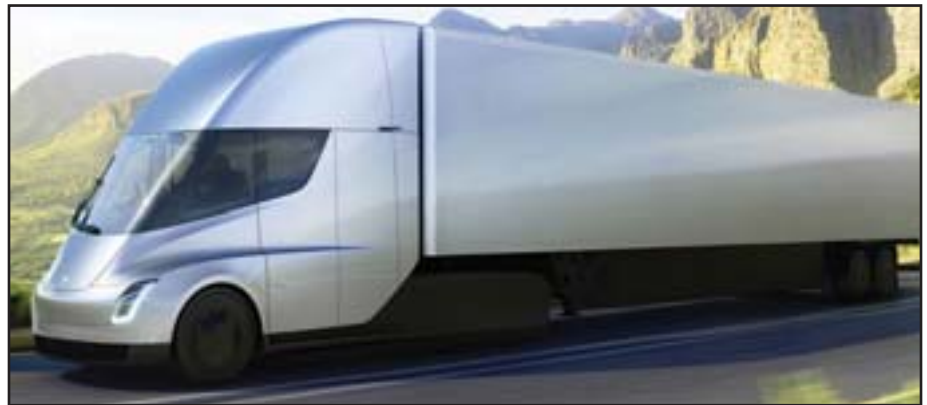
The Tesla electric semi-truck gives the freight industry an electric option. The truck can have a range up to 500 miles.
